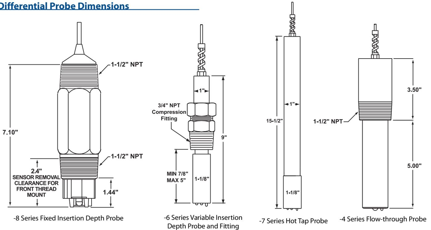
The Aquametric family of differential probes includes the fixed insertion -8, the variable insertion -6, an extended length version of the -6 for hot tap connections—the -7 and the flow-through version -4.
