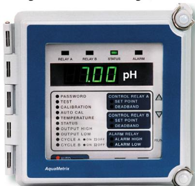
The 2200 controllers feature a large bright LED display and intuitive user interface packaged in a NEMA 4X fiberglass enclosure. Frequently used functions are accessed through an intuitive step-through menu printed directly on the front panel. Seldom used adjustments such as the temperature unit are set using DIP switches on the back of the swing-out front panel.
