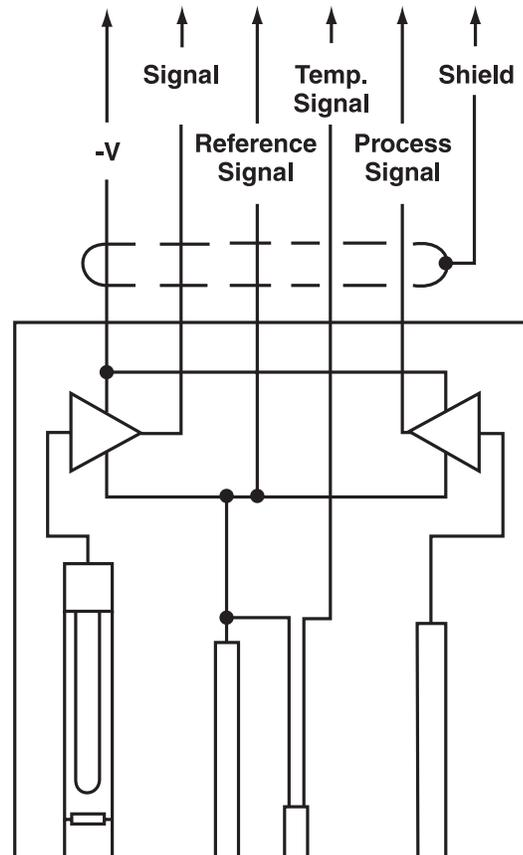
*The advantage of differential pH measurement is shown here. The signals from both process and reference electrodes subtract out the signal of the ground (or return) electrode which measures any non-zero or varying ground voltage. In addition, the separation of the two electrodes allows both the salt bridge connecting the two and the pH 7 buffer solution in which the reference electrode sits to be replaced.*
