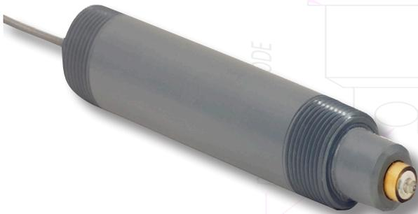
The P575 Combination probe features a combination glass electrode encapsulated in epoxy and housed in a CPVC body with 1" NPT threads on both ends.
