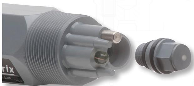
Exploded view showing the salt bridge and the well containing the reference electrode. Both the salt bridge and buffer solution can be replaced at little cost.
